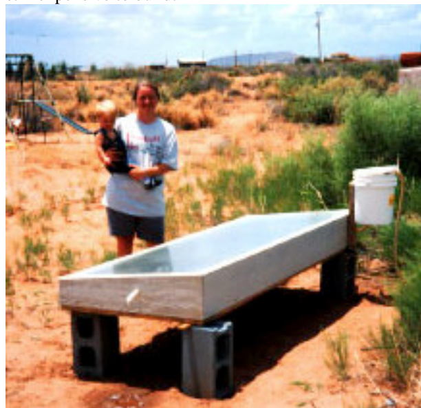
Fig. 2. First generation concrete sided EPSEA solar still built in 1995 that has been operational for over a decade for the Eby family in Hueco Tanks, Texas. This still uses a food grade rated silicone membrane.
